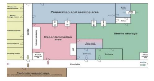
**Fig 5.7** Suggested design of a Sterile Supply Department. Please note the flow of devices and staff from clean to dirty areas to avoid recontaminations of items and instruments.
